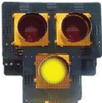
Solid Yellow The flashing yellow is followed by a SOLID YELLOW signal, indicating drivers should reduce speed and be prepared to stop.
